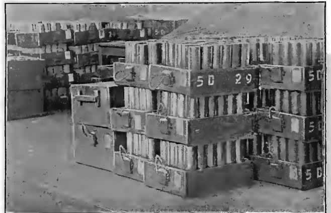
FIG. 4. TOTE BOXES USED FOR TRANSPORTING BRASS CARTRIDGE CASES
